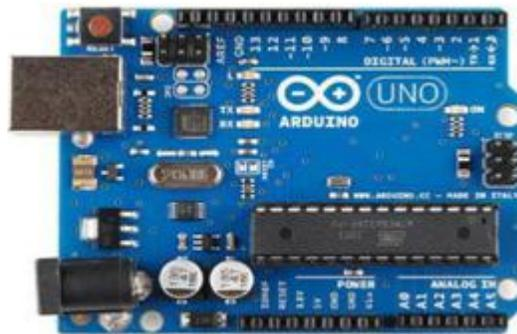
*Figure: Arduino Microcontroller*
